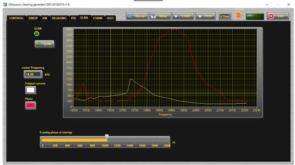
11. Press the SCAN button. The scanning procedure starts. There is a drawing consisting of phase characteristic (red line) and current characteristics (white line). It should be similar to the picture with well-defined phase feature. This diagram shows the actual operating parameters of the transducer. If necessary, pick new Fstart and SPAN (in CONTROL tab).
