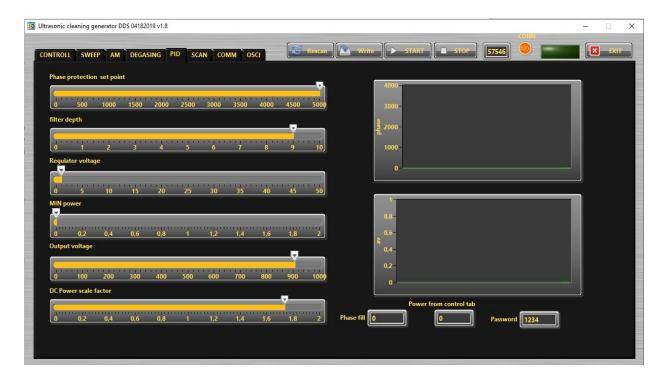
Phase Protection Set Point – If everything is normal and normal work of the transducer, the operating phase will be 2000-2500 units. If the transducer works on air(no load) the phase will increase 3000 units and higher. Use this as a protection against "No load operation" to save the transducer.
